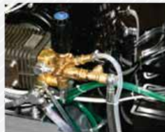
Pressure regulator and safety valve
